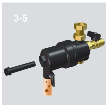
Removing the magnet (turn it 90° clockwise)
